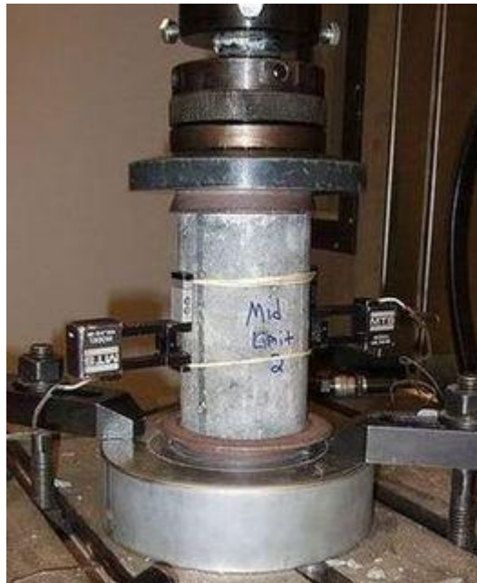
Figure 2: Compressive Strength Testing of Algae-Based Concrete Specimens at 28 Days
