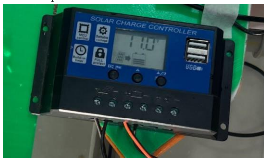
Fig[4] MPPT Solar charge controller charging the battery
