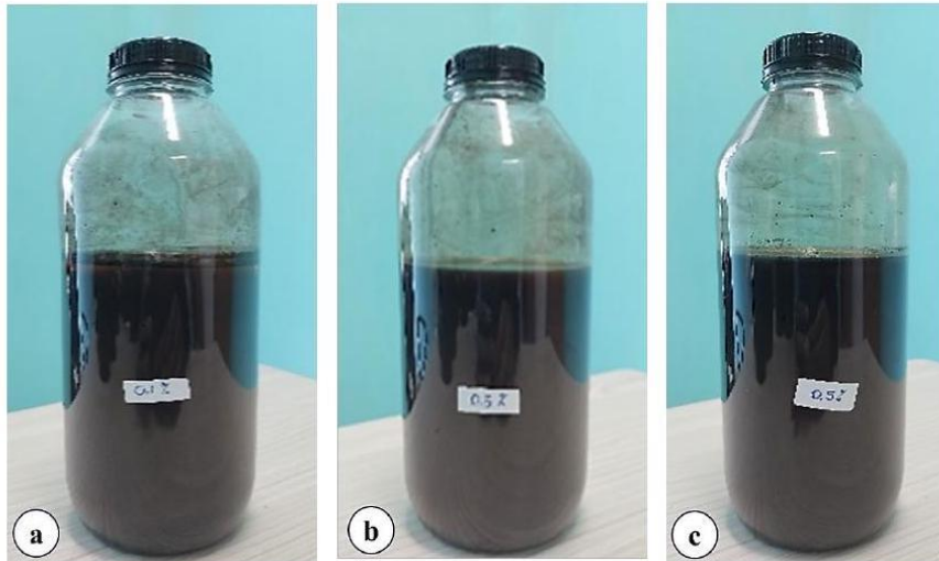
Figure 3. CuO nanofluid: (a) NF 0.025%, (b) NF 0.055%, and (c) NF 0.102%
