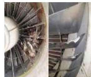
Fig.6.6: Bird strike engine damage
