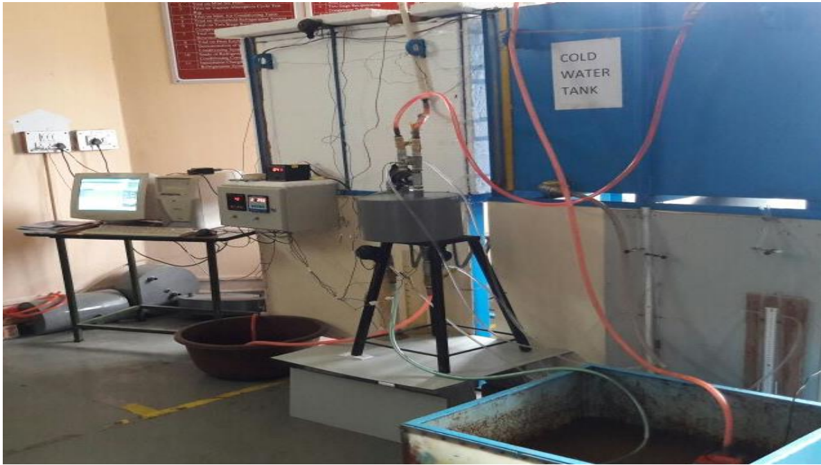
Fig. 2.2: Photograph of experimental set up of helical cone coil heat exchanger
